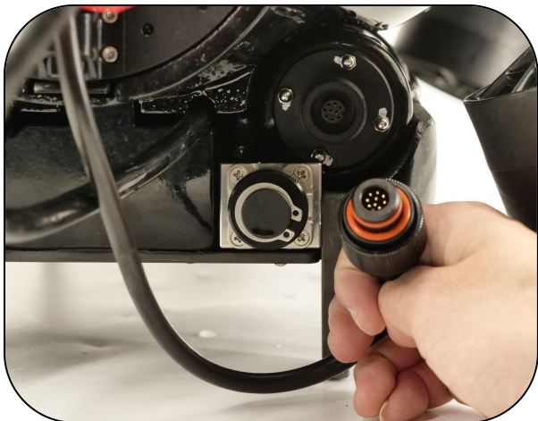
3.2.2.2 Connect the communication cable on the ROV to the type-A Q-interface
